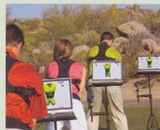
In a K-Vest class, golfers get instant swing feedback via sensors that transmit data to a computer.
