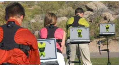
Sensors placed at the top and bottom of the spine and on the glove hand combine to give golfers feedback on swing sequence and body movement. (courtesy photo)
